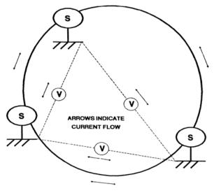
Figure 2 – Ring LAN Showing Ground Loops
