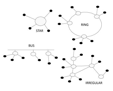
Figure 1 - Typical Hard-wired LAN Topologies
