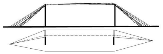
Figure 4 – Typical Bounded Wave Simulator
